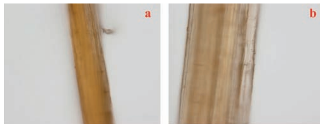
Figure 3. Optical micrographs of acrylated broom fibers copolymerized with (a) a stoichiometric amount of DMAA and (b) an excess of DMAA.
